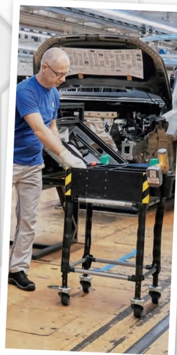
Synchronously running cart: The necessary tools and materials are always within reach for employees.
