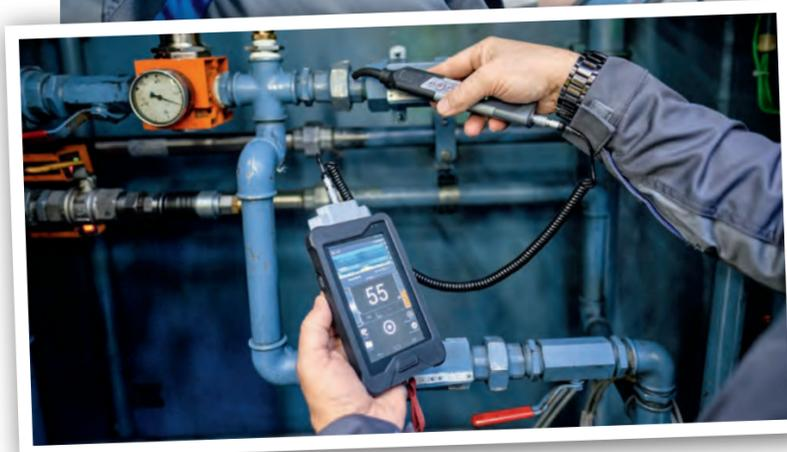
Measurement: Leaking air can be detected with a digital ultrasound device.
