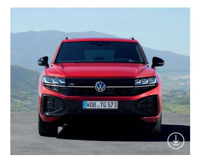
A horizontal white LED strip in the radiator grille is part of the daytime running lights of the IQ.Light HD matrix headlights.
